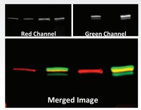
**Figure 6.** Multiplexing on a single blot is a unique method available with digital imagers. Here, a western blot has been probed for both STAT1 (red channel) and phosphorylated STAT1 (green channel) using fluorescently conjugated secondary antibodies and imaged using infrared detection on the Azure c600. This information would involve many more steps and much more time using film.
