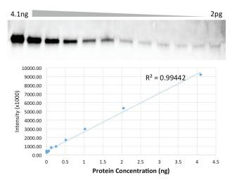
**Figure 3.** Digital images offer signal linearity, increased dynamic range, and a low limit of detection. The chemiluminescent signal on a western blot of a serial dilution of transferrin was imaged on an Azure c600. Quantitation of the bands demonstrates a linear signal with a dynamic range over three orders of magnitude and a limit of detection of 2pg.
