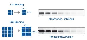
**Figure 2.** Binning is a powerful technique for digital imaging of chemiluminescent western blots. Binning increases sensitivity by combining pixels to make a larger, extra sensitive pixel with a better signal to noise ratio.
