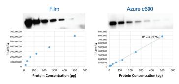
**Figure 5.** An illustration of the difference in linearity between a digital image and x-ray film. For accurate quantitation, signals must be within linear range of each other – the bright signals from the film are saturated and no longer linear. The same blot was imaged on both Lucent Blue X-ray Film and the Azure c600 for 1 minute, and the correlation between the signal and protein concentration is indicated in the two diagrams.
