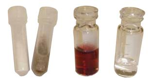
Figure 1: Top: dSPE tubes with 150mg MgSO $_4$  and 150mg PSA before and after cleanup of 1mL red wine extract; Bottom: Red wine extract before and after dSPE cleanup.
